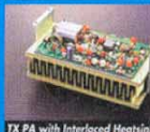
TX PA with Interlocked Heatsinks
